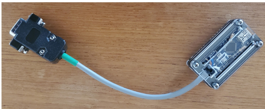
W0YK homebrew hardware for TinyFSK (“ Mortty Version 0”).
